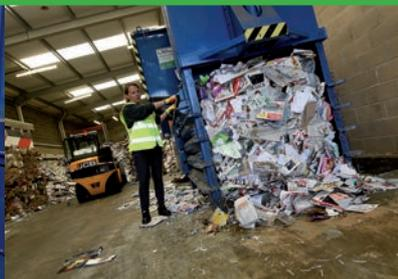
A finished paper bale is wired and removed from the baler ready for shipping.
